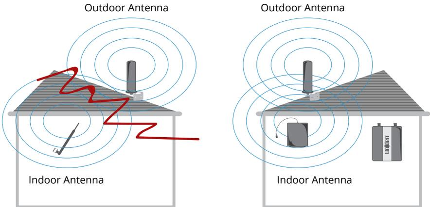
The indoor antenna is pointed at the outdoor antenna. The antennas are too close together
