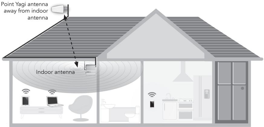
Oscillation is caused when the indoor (distribution) antenna sends a signal back into the outdoor (signal) antenna. Similar to a PA system, when the microphone gets too close to the speaker it causes feedback. This will occur if your antennas are too close together, or the indoor antenna is pointed at the outdoor antenna. Make sure you have adequate separation and some types of shielding between the antennas (usually your roof or a cement wall is good enough).
